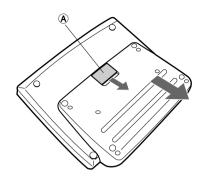
When the player is not used for an extended period of time, disconnect the battery pack from the unit. When it is connected, a small amount of current continues to flow to the player, even when the power is turned off. If left connected for a long time, the battery may become over-discharged.
